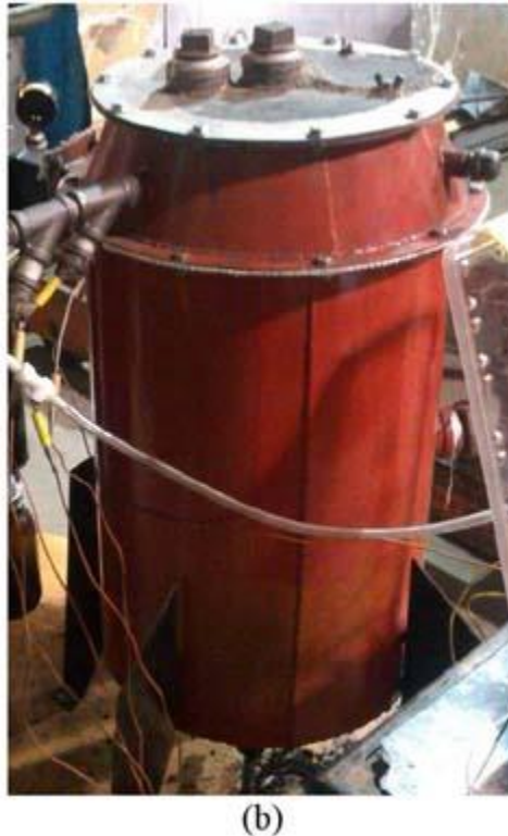
Figure 2 (a) A schematic of down draft gasifier and different stages happen during the process (b) A pilot-scale GEK gasification reactor ( Foley and Barnard )
