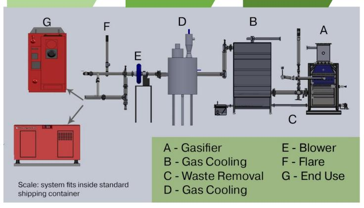
The bioHearth® downdraft gasification system is the simple, affordable waste to energy solution.
